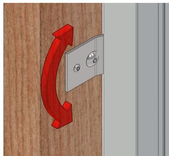
The straps must be securely screwed to the door frame and welded or screwed to the wall.
